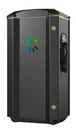
**Charging Mode** Mode 3 Socket or Tethered Lead AC Output Current (A) 6,10,16,20,25,32 Power outlet [kW] 3.7KW,7.4KW Rated voltage [V AC] 230 / 400 Frequency [Hz] 50 -25...+40 Temperature range [C] Degree of protection (IP) 44
